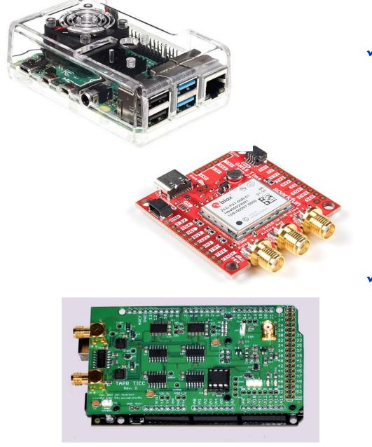
Idea C could be implemented with about \$600 USD of hardware, plus the cost of a chassis and connectors. For purposes of example, the CPU could be a Raspberry Pi (\$100), the TIC the TAPR unit with 60 ns resolution (\$200), and the GPS unit a development board based on the multi-constellation, multifrequency uBlox F9T (\$300).
