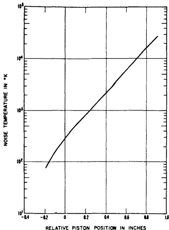
Fig. 10. Calibration curve of comparator.
