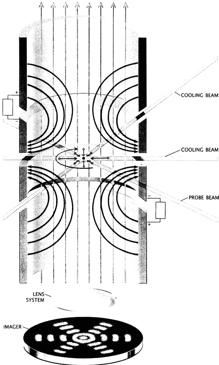
**PENNING TRAP** generates electric fields (*red lines*) and magnetic fields (*green lines*) to produce forces (*black arrows*) that confine charged particles. The electric and magnetic fields also cause the microplasma to rotate. Two laser beams cool the particles; a third serves as a probe for various experiments. The magnetic field arises from an electric current flowing through a solenoid (not shown) that encircles the trap.
