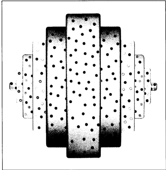
**SHELL STRUCTURE** of a microplasma consisting of about 1,000 beryllium ions is revealed in a photograph (*left*) made by shining a laser beam through the microplasma and recording the resulting fluorescence. The illustrations depict the complete
