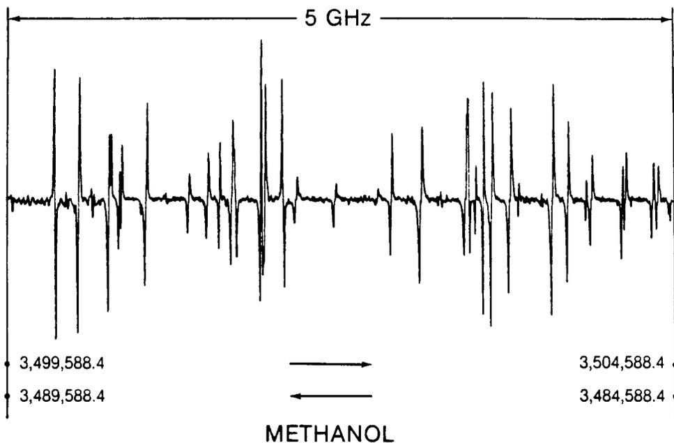
Figure 3 : A far infrared scan of methanol: a pressure of about 10 Pa of methanol and a frequency modulation of 2.5 MHz were used to record the spectrum. Both sidebands are shown: the lines which are positive on the left are those in the increasing frequency sideband and vice versa for those which are negative on the left. The frequencies are in megahertz.
