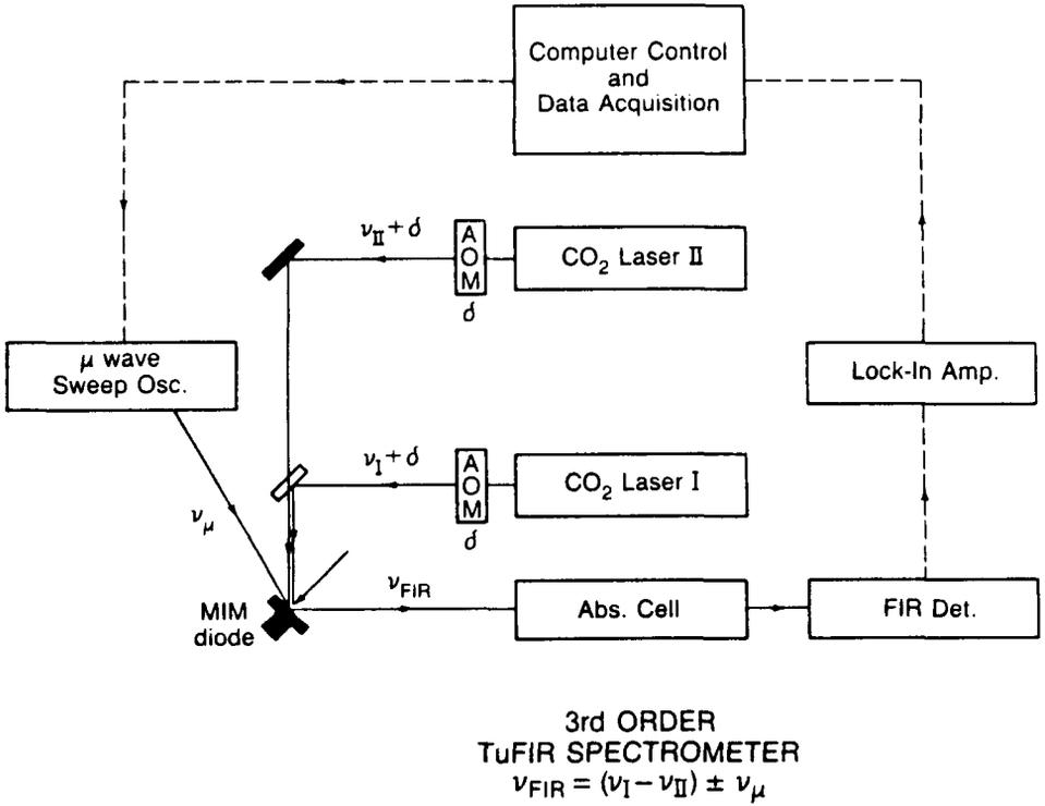
Figure 2 : The Third Order Tunable Far Infrared Spectrometer.
