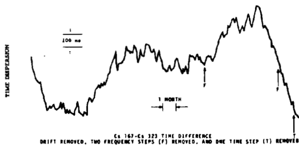
Fig. 18 - Random time fluctuations of Cs 167 - Cs 323 after removal of frequency drift, 2 F-steps, and 1 T-step.
