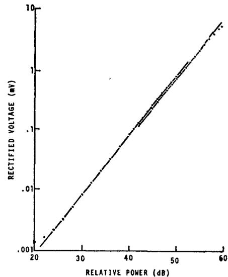
Fig. 6. Response of diode used as detector: rectified dc voltage versus microwave power.
