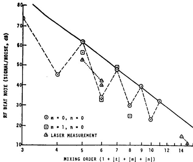
Fig. 1. RF beat note (S/N) versus mixing order for microwave signals at 20 GHz and laser signals at 3–11 THz. No bias voltage was used.
