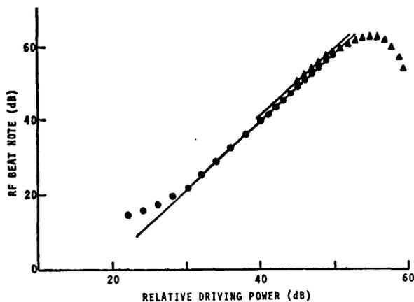
Fig. 5. RF beat signal generated by two microwave oscillators as a function of the lower frequency microwave oscillator power.
