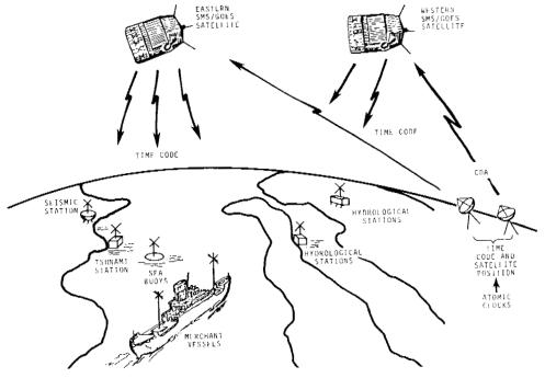
Fig. 13-Illustration of SMS/GOES time code distribution
