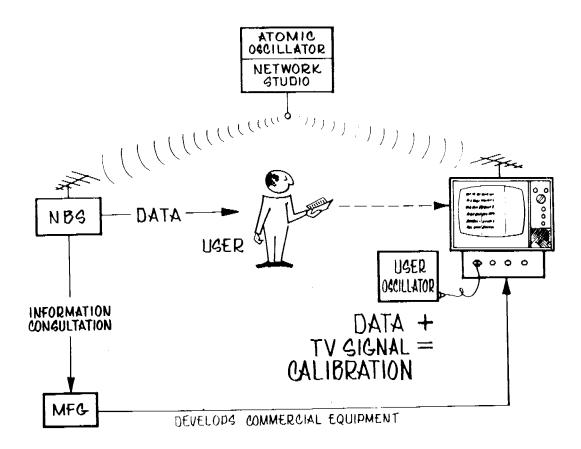
Fig. 6-TV frequency calibration service
