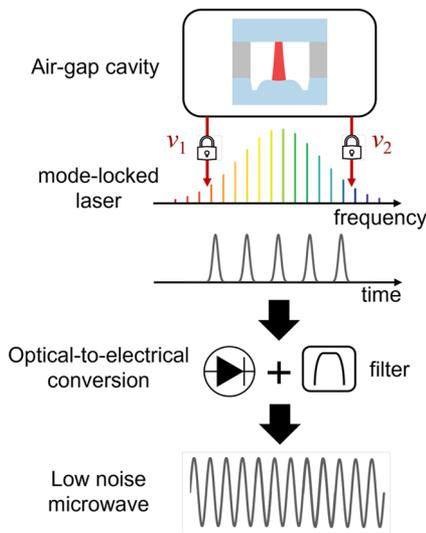
**FIG. 1.** Conceptual diagram of 2-point optical frequency division with an air-gap optical reference cavity. Two lasers locked to the same air-gap cavity are used to stabilize the repetition rate of a mode-locked laser. The fractional frequency stability of the generated microwave inherits the stability of the cavity free spectral range.
