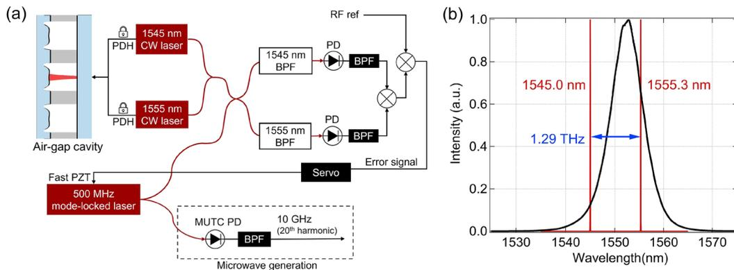
**FIG. 4.** (a) Schematic diagram of 2-point lock microwave generation with the air-gap cavity. The mode-locked laser repetition rate is stabilized via feedback to a fast piezoelectric transducer (PZT). PDH: Pound–Drever–Hall lock; BPF: bandpass filter; and MUTC PD: modified uni-traveling carrier photodiode. (b) Optical spectrum overlap between the mode-locked laser (black) and CW lasers (red).
