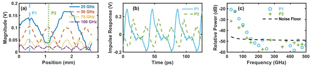
Fig. 2. Measurements of voltage standing waves along the CPW. (a) Magnitude of the voltage waves at 25 GHz, 50 GHz, 75 GHz, and 100 GHz versus sampling position ( $40\ \mu\text{m}$  pitch) along the CPW. (b) Reconstructed time domain waveforms at locations marked P1 and P2, showing the effect of spatially dependent impedance along the CPW terminated by an open circuit. (c) Corresponding frequency content and estimated noise floor at P1 and P2.
