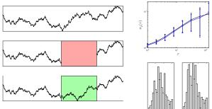
Fig. 3. Application of data imputation algorithm on simulated data of the four predominant noise types. Left: The data reconstruction algorithm. On the top left is the original data, in the middle left the dataset with values removed, and on the bottom left the dataset with imputed values. Top Right: The Allan deviations for the original (black) and recovered (blue) datasets. Bottom Right: The distribution for the original is in the left box and for the recovered data is in the right box.
