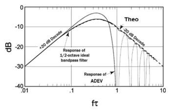
Fig. 1. Digital frequency filter of Allan variance (AVAR), hence, its squareroot ADEV. Also shown is Theo1, a statistic created to eliminate the nulls of standard ADEV and match the ideal bandpass response of two cascaded filters, a single-pole high-pass followed by a low-pass with identical break points at  $RC = \tau/2$  (dashed line).
