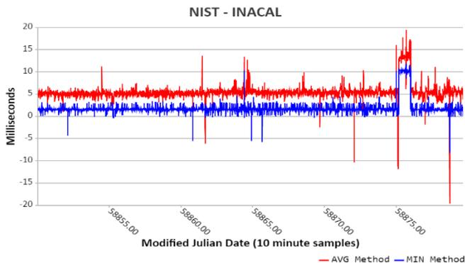
Fig. 3. Comparison during 30 days of the NTP Server of the Time and Frequency Laboratory of INACAL with respect to NIST.
