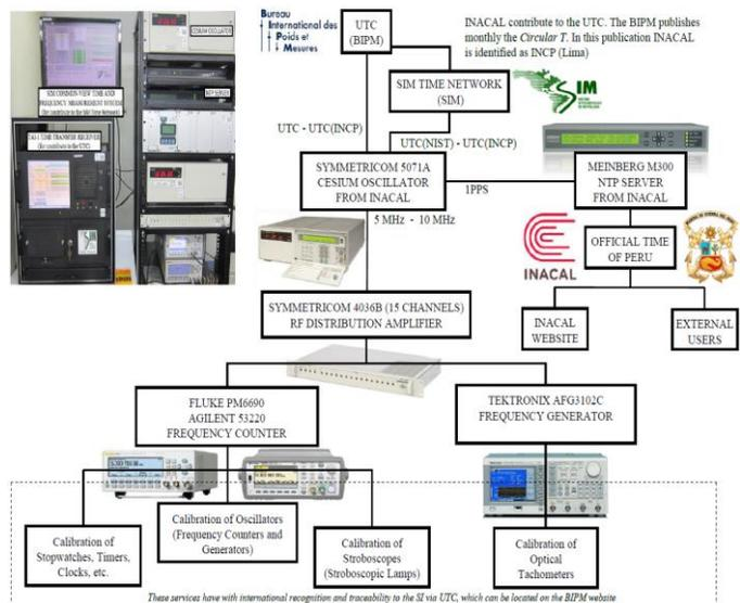
Fig. 4. Traceability chain of the Time and Frequency Laboratory of INACAL.
