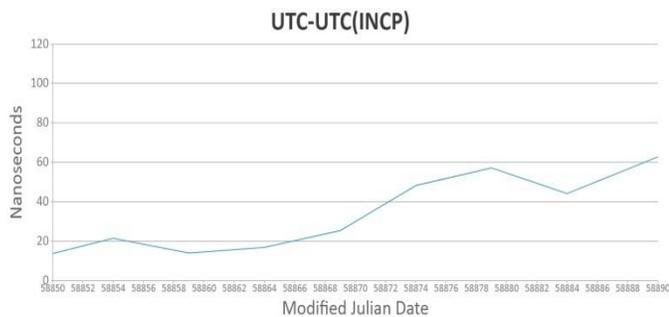
Fig. 2. Comparison during 40 days of the standard oscillator of the Time and Frequency Laboratory of INACAL with respect to UTC.
