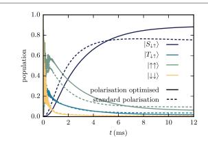
**Figure 5.** Time-dependent population in the states  $|\downarrow\downarrow\rangle$ ,  $|\uparrow\uparrow\rangle$ ,  $|S_{\downarrow\uparrow}\rangle$  and  $|T_{\downarrow\uparrow}\rangle$  after summing over all motional levels. The graph compares the dynamics when starting with all population in the  $|\downarrow\downarrow\rangle$  state initially, before (dashed lines) and after (solid lines) the combined optimization, leading to fidelities of F=76% and 88%, respectively.
