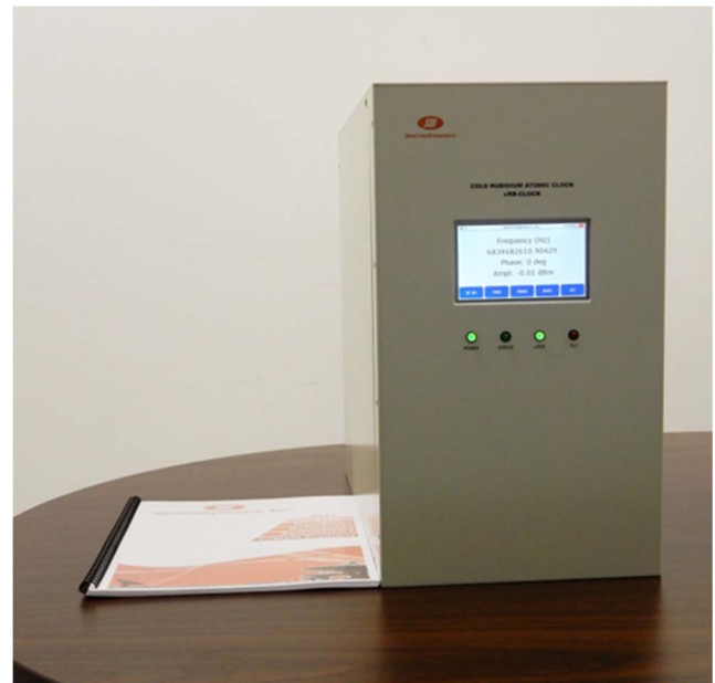
Figure 1 – Prototype of the portable cold Rb87 atomic clock. The clock is packaged in a 22 X 37 X 32 cm enclosure and weighs about 28 kg. The signal and power connections are on the rear panel of the instrument.
