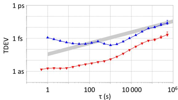
FIG. 5. Time deviation (TDEV) of the optical pulse-train timing comparison (red down-pointing triangle) and the 1 PPS timing comparison (blue up-pointing triangle) over 37 days. The gray region represents the best possible TDEV supported by current optical clocks [32,33]. Values have been divided by  $\sqrt{2}$  assuming equal contribution from each comb.
