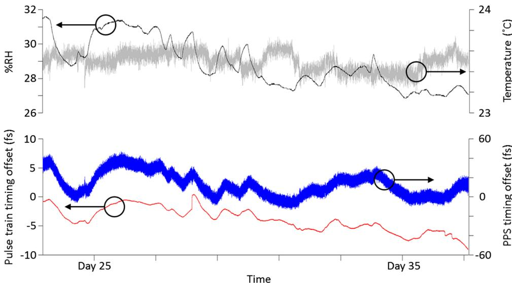
FIG. 3. Top panel: Relative humidity (%RH) (black) and temperature (gray) data for the last two weeks of timing comparison experiment during which humidity data were available. Temperature data have been smoothed with a 10-min window. Bottom panel: Pulse-train timing (red) and PPS timing (blue). The strong correlation between humidity and timing offsets is clearly evident.
