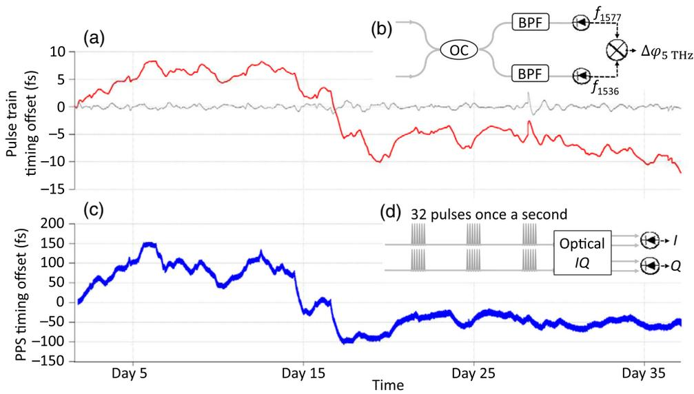
FIG. 2. (a) Time offset between the two optical pulse trains (red line) as measured for 37 days using the synthetic wavelength technique. After high-pass filtering (gray line) the data show the clear absence of phase slips. (b) Setup of the pulse-train optical timing comparison. BPF, optical band-pass filter. (c) Time offset between the PPS clock outputs (blue line) over the same 37-day period. (d) Setup of the PPS optical timing comparison.
