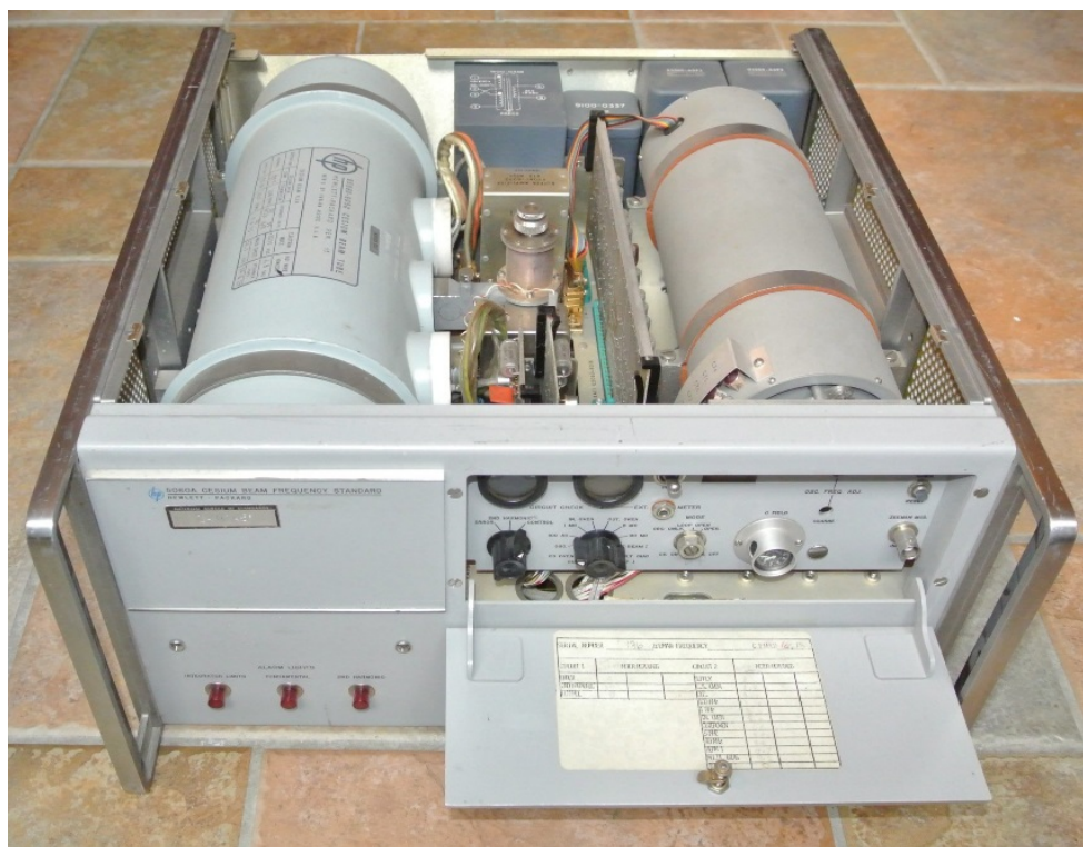
Fig. 9. Hewlett-Packard 5060A cesium beam atomic clock with cover removed showing beam tube on left (courtesy of Tom Van Baak, leapsecond.com).
