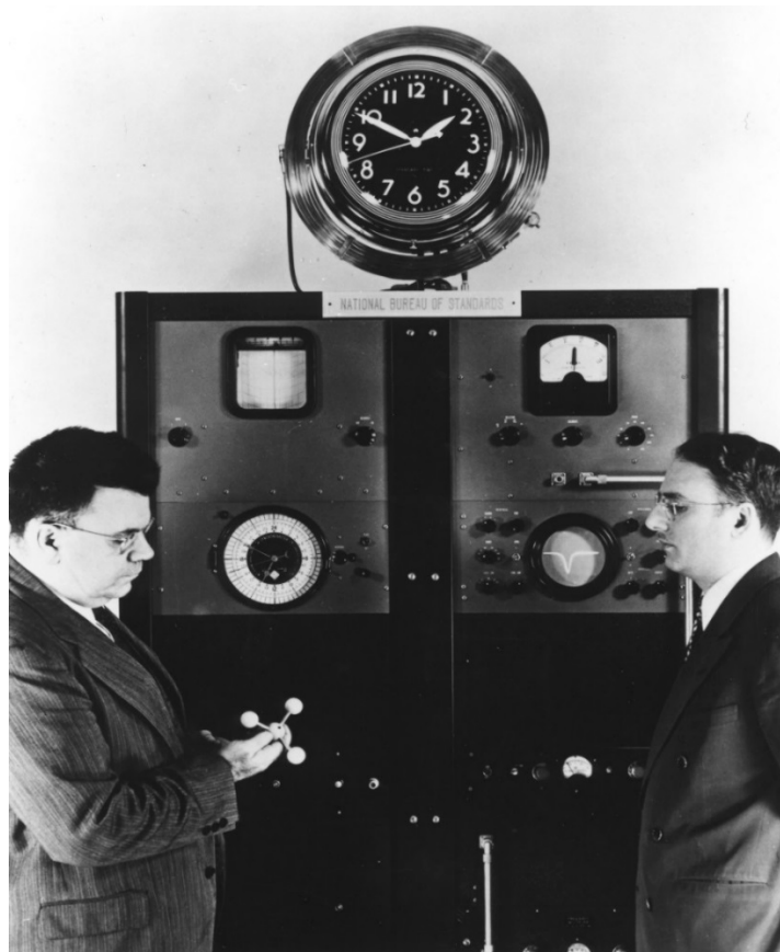
Fig. 2. Dr. Harold Lyons (right), inventor of the ammonia absorption cell atomic clock, observes, while Dr. Edward U. Condon, the director of the National Bureau of Standards, examines a model of the ammonia molecule (1949). The clock atop the equipment racks was driven by a 50 Hz signal obtained by dividing the signal from a quartz oscillator that was locked to the ammonia absorption frequency. However, its primary function was to let the world know that the invention was indeed a clock.
