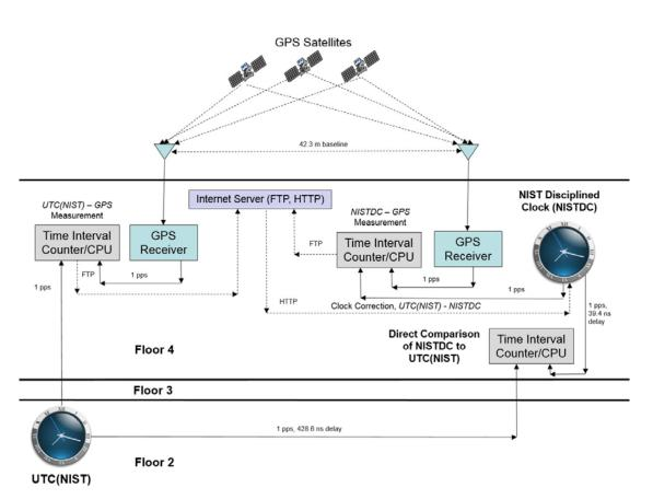
Fig. 8. Measurement configuration for direct comparison of a NISTDC to UTC(NIST).
