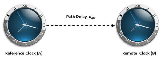
Fig. 3. A simple "one-way" time transfer system.
