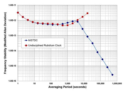
Fig. 7. Comparison of frequency stability of NISTDC to undisciplined rubidium clock, with respect to UTC(NIST).
