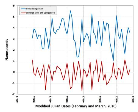
Fig. 9. Direct and Common-View Comparisons of a NISTDC at NIST prior to shipment.
