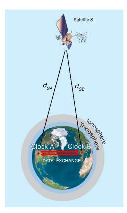
Fig. 4. Common-view time transfer via satellite.
