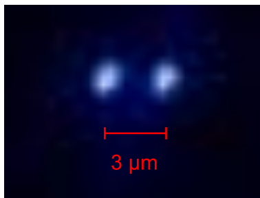
Figure 9. EMCCD image of two trapped ^{25}\text{Mg}^+ ions loaded into a surface-electrode RF-Paul trap.
