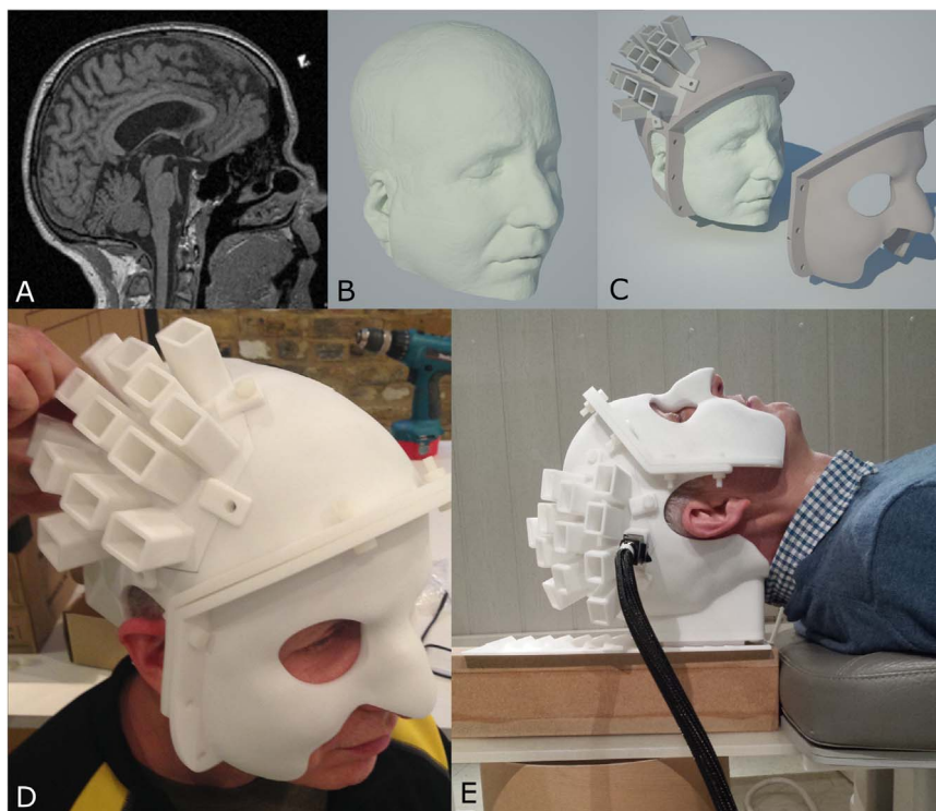
Fig. 2. Head-cast design and fabrication: A) Single sagittal slice from the anatomical MRI. B) Outer head surface extracted from MRI. C) CAD model of the head-cast with slots designed to house the OPM sensors over sensorimotor cortex. Slot positions are based on a-priori prediction of the spatial topography of scalp field pattern, derived from previous SQUID measurements in the same subject. D) 3D-printed head-cast on subject. E) Subject in situ with the OPM attached. Note that the head-cast is not only fixed rigidly to the subject's scalp, but is also fixed relative to the MSR, thus eliminating any sensor motion relative to the subject, and subject motion relative to the MSR.
