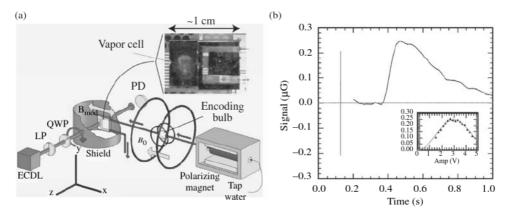
Figure 7.8 (From Ledbetter et al. [45].) Measurement of weak nuclear polarization in water by use of a microfabricated atomic magnetometer. (a) Experimental setup showing tap water running through 8cec619 a polarizing magnet and onto the NMR detection chip. (b) Change in the signal observed by the magnetometer after application of a  $\pi$ -pulse in the encoding bulb at the time indicated by the vertical line.
