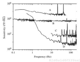
Figure 7.6 Sensitivity of microfabricated atomic magnetometers. (A) Integrated coherent population trapping magnetometer (Schwindt *et al.* [35]), (B) integrated  $M_x$  magnetometer (Schwindt *et al.* [14]), (C) SERF magnetometer in microfabricated vapor cell (Shah *et al.* [1]), (D) advanced SERF magnetometer in microfabricated vapor cell (from Griffith *et al.* [21]).
