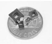
Figure 7.5 A variety of microfabricated alkali vapor cells, showing a range of interior dimension from 4 mm to 0.5 mm.
