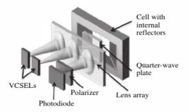
Figure 7.3 Reflectors internal to the cell can be used to redirect laser beams and create perpendicular pump/probe geometries.
