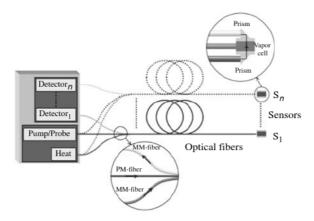
Figure 7.4 Concept of fiber-optically coupled magnetometer array. A series of sensor heads  $(S_1 - S_n)$  is coupled fiber-optically to a common control unit containing a pump/probe laser, a heating laser, and a series of photodetectors.
