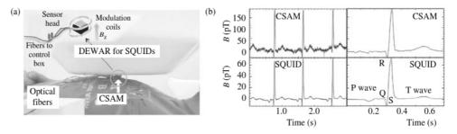
Figure 7.7 (From Knappe et al. [40]. Copyright 2010, American Institute of Physics.) Measurement of the magnetic field from a human heart by use of a microfabricated atomic magnetometer. (a) Experimental setup showing a microfabricated atomic magnetometer (CSAM) positioned below a SQUID dewar. (b) Measurements were made simultaneously with a SQUID sensor for comparison.
