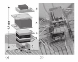
Figure 7.2 (Adapted from Ref. [14].) (a) Design and (b) photograph of a chip-scale atomic magnetometer. A laser (1), surrounded by a spacer (2), emits light through some optics (3) to illuminate a Sec 619 vapor cell (5); the light is detected with a photodiode (6). Ohmic heaters (4) are used to heat the cell.
