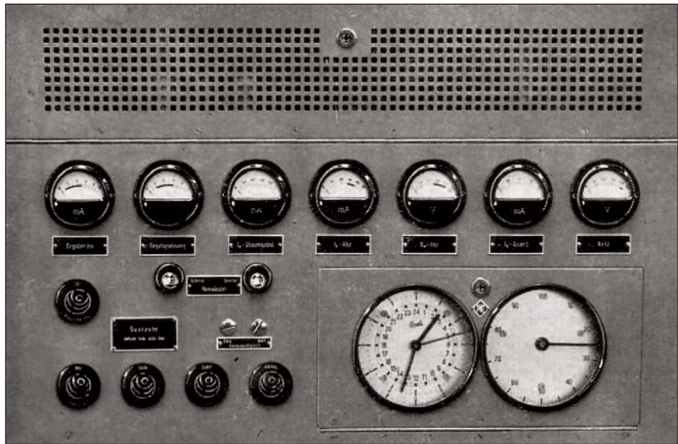
Fig. 7. Rohde & Schwarz Model CFQ, the first portable quartz crystal clock (courtesy of Rohde & Schwarz).
