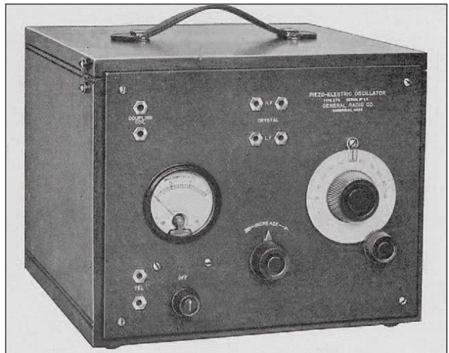
Fig. 4. The first commercial quartz oscillator, the General Radio Type 275.
