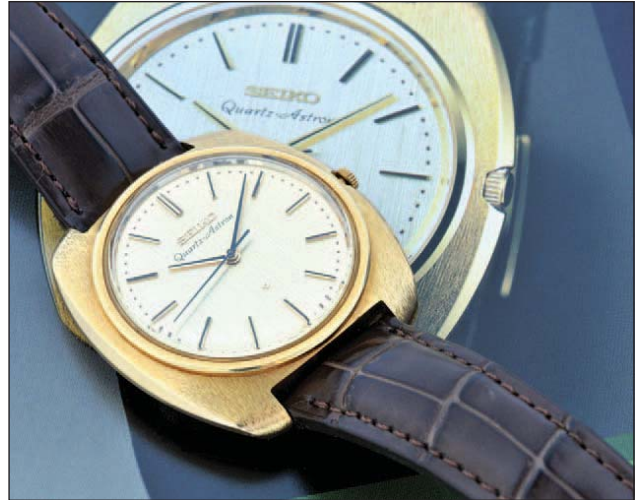
Fig. 9. The first commercial quartz watch, the Seiko Astron (courtesy of Seiko).
