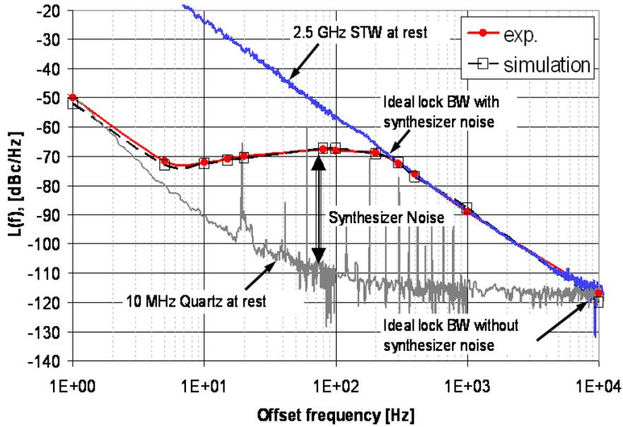
Figure 2. Measured and simulated PM noise of the combined 2.5-GHz and 10-MHz quartz (scaled to 2.5-GHz) oscillators at rest with the scheme shown in Figure 1(a). The frequency synthesizer noise is included.  $L(f)$  — single-sideband PM noise.
