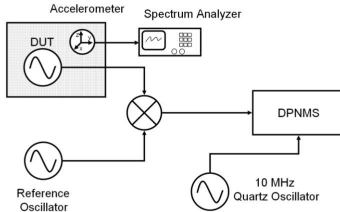
Figure 3. Setup for measuring PM noise and vibration sensitivity of oscillators. DPNMS — Direct digital phase noise measurement system.
