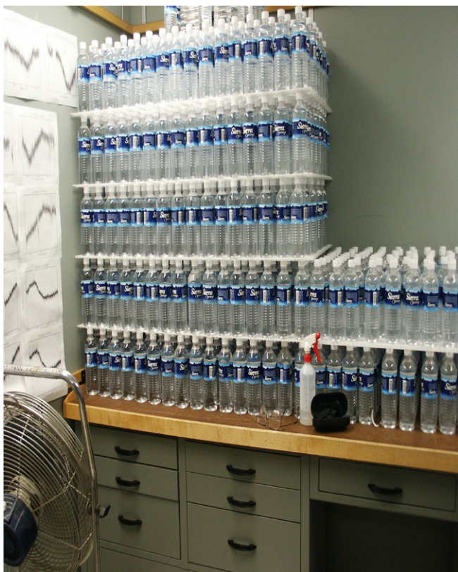
Figure 9. A portion of the water bottles added to the time scale room to stabilize its temperature. The water attenuates the short-period fluctuations, but has little effect on the long-period and seasonal fluctuations.
