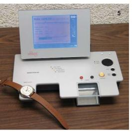
here, the mechanical quartz oscillations are acoustically recorded. The device can also capacitively record the stray electrical field from quartz oscillators with open movements or with cases made of synthetic material. It is also possible to derive the quartz frequency from the supply current if the analyser is providing power to the watch.<sup>6</sup>
