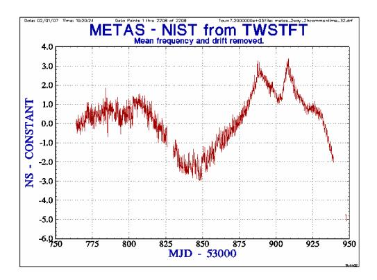
Figure 5. METAS-NIST time-transfer values obtained from TWSTFT 29 Jan - 31 Jul 2006 (drift and frequency offset removed). The diurnals in the TWSTFT values grow smaller as winter becomes spring, with a noticeable transition around MJD 53875.
