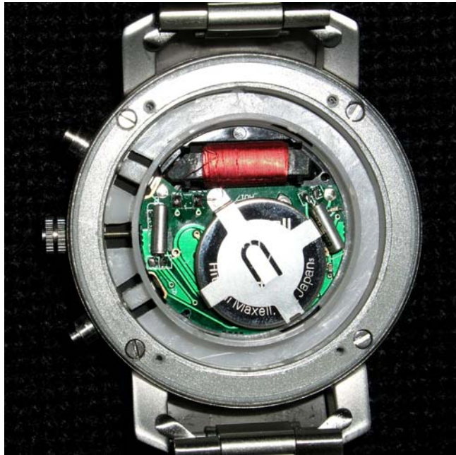
The interior of a low cost watch controlled by WWVB signals. Note the ferrite bar antenna at the top of the movement and the two encapsulated crystal oscillators below, one on each side. One a 32.768 kHz crystal that drives the quartz clock, the other is a 60 kHz crystal that serves as a preselector for the time signal. The battery appears to take up more area than the crystals and antenna combined.
