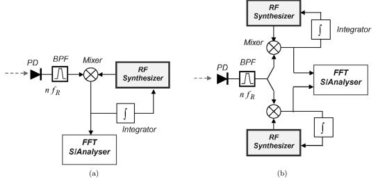
Fig. 1. Single-channel (a) and dual-channel (b) two oscillator phase noise measurement systems.
