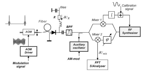
Fig. 3. Experimental setup for measurement of power-to-phase conversion in photodetectors.
