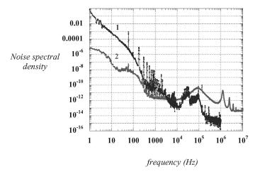
Fig. 2. Spectra of phase (curve 1) and amplitude (curve 2) fluctuations of a signal at second harmonic of pulse repetition rate at the output of a photodetector illuminated with a Cr: forsterite femtosecond laser. The units of the vertical axis are rad<sup>2</sup>/Hz for the phase noise and 1/Hz for the amplitude noise, respectively.
