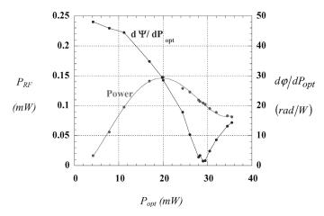
Fig. 4. Power of second harmonic of pulse repetition rate (866 MHz) and power-to-phase conversion at the same frequency as a function of average power of the optical comb. "Discovery" photodetector, load resistor 100  $\Omega$ , bias voltage 6 V.
