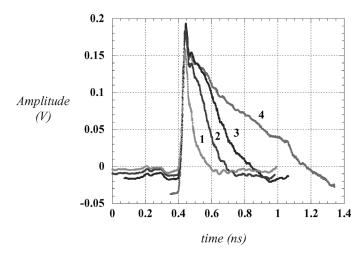
Fig. 6. Demodulated light pulses at the output of "Discovery" photodetector at different levels of optical power (photocurrent): curve 1, photocurrent  $I_{DC}=1.1$  mA; curve 2, photocurrent  $I_{DC}=3$  mA; curve 3, photocurrent  $I_{DC}=5$  mA; curve 4, photocurrent  $I_{DC}=11$  mA. Photodetector is directly connected to a matched input of a high-speed oscilloscope.
