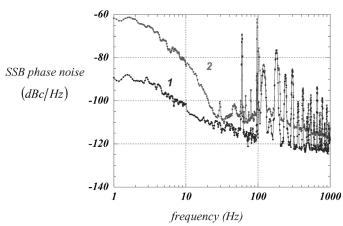
Fig. 11. Effect of power control system on the excess phase noise in the spectrum of the second harmonic of pulse repetition rate: control system is activated (curve 1), control system is off (curve 2). Photocurrent is 11.4 mA.
