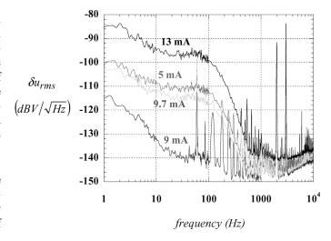
Fig. 8. Spectra of voltage fluctuations at the output of the external channel of the dual-channel phase sensitive read-out system at different levels of photocurrent. Measurements were carried out with two "Discovery" photodetectors at the frequency 866 MHz which is the second harmonic of pulse repetition rate. Bias voltages were set to 6 V, the load resistances were 100 ohm.
