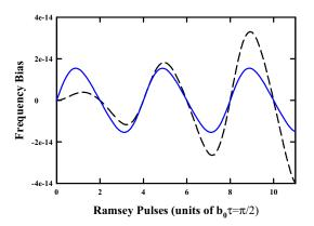
Figure 5. The modeled frequency bias induced by leakage below the Ramsey cavity. The solid curve is the case where the leakage amplitude is constant while the field in the Ramsey cavity is increased. The broken curve is the case where the leakage field amplitude is proportional to the amplitude of the field within the Ramsey cavity. In both cases the microwave power level has been chosen purely for convenience and has no particular significance.
