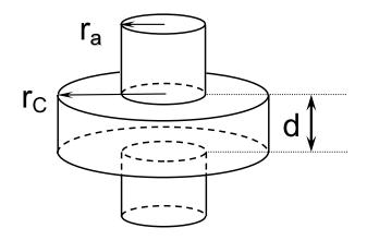
Figure 1. A schematic diagram of the  $TE_{011}$  microwave cavity used in most cesium fountain frequency standards.
