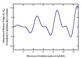
Figure 2. The distortion of the Ramsey fringe plotted caused by distributed cavity phase with respect to the microwave excitation (number of  $\pi/2$  pulses). The distortion is proportional to the frequency bias and the data shown here are normalized to the shift at optimum power (one  $\pi/2$  pulse).
