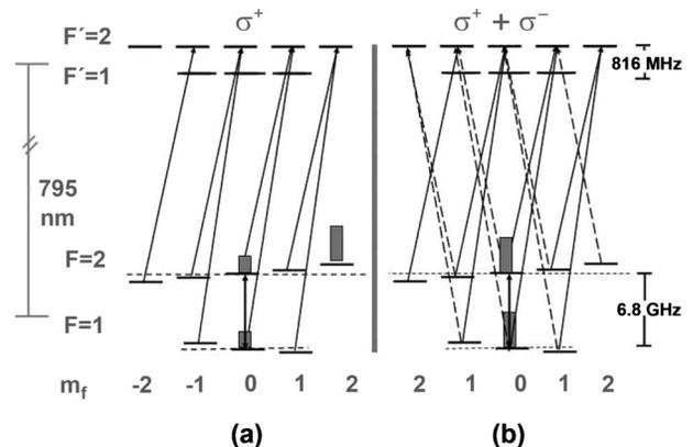
Fig. 1. (a)  $\sigma^+$  polarized light fields incident on the  $D1$  line of  $^{87}\text{Rb}$  in  $\Lambda$  configuration. A large fraction of atoms is lost to the  $|F=2, m_f=2\rangle$  state, resulting in a loss of CPT resonance signal. (b) A combination of  $\sigma^+$  and  $\sigma^-$  light fields can be used to accumulate a maximum number of atoms in the CPT dark state on  $m_f=0:0$  ground states.
