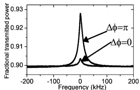
Fig. 3. CPT resonances for two values of relative modulation phase  $\Delta\phi$ .
