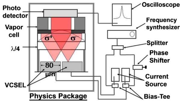
Fig. 2. (Color online) Schematic of the experimental setup. The proposed technique is experimentally implemented in a highly miniature physics package.
