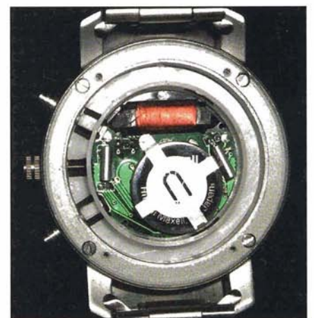
The interior of a low cost watch controlled by WWVB signals. Note the ferrite bar antenna and two crystal oscillators, one a 32,768 kHz crystal that drives the quartz clock, the other is a 60 kHz crystal that serves as a pre-selector for the time signal. The battery appears to take up more area than the crystals and antenna combined.
