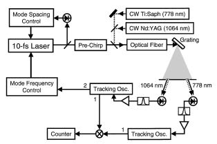
Fig. 1. Block diagram of the apparatus used for measurement of the 104-THz gap between 1064 and 778 nm. Osc's, oscillators.
