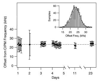
Fig. 3. Summary of measured Nd:YAG frequency  $f_{1064}$  with respect to the CIPM recommendation of 281, 630, 111, 740 kHz. The dashed line is the average of all the plotted points (23.2 kHz). The inset is a histogram of the ~800 individual measurements on and after the third day.
