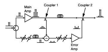
Fig 5. Block diagram of a feed-forward linear amplifier. Two-tone intermodulation byproducts are shown in the power spectra at various points in the diagram.
