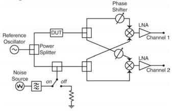
Fig 2. Block diagram of PM noise-measurement system for amplifiers. LNA is "low noise amplifier" and DUT is "device under test."
