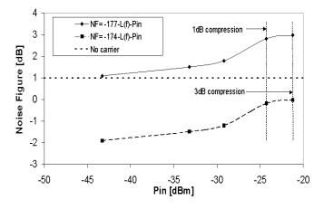
Fig 3(b). Variation of NF with input power for the amplifier in figure 3(a).
