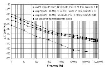
Fig 7. Variation of flicker noise of different amplifiers with Fourier frequency at 10 GHz.
