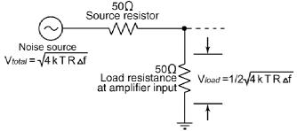
Fig 1. Equivalent input circuit showing the thermal noise generator with a source resistance of 50  $\Omega$  terminated with the amplifier's input (load) resistance, which is also 50  $\Omega$ . Note that the thermal noise voltage is divided in half at the amplifier's input (maximum power transfer theorem).
