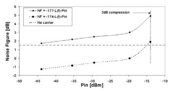
Fig 4(b). Variation of NF with input power for the amplifier in figure 4(a).
