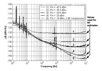
Fig 4(a). PM noise of GaAs FET amplifier at different input power levels. Gain= 35 dB, NF= 1.5 dB, frequency= 10 GHz.
