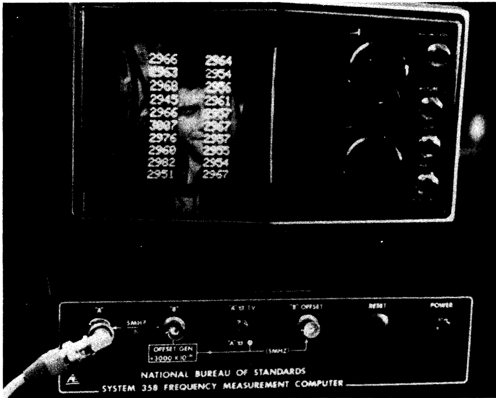
FIGURE 7.5. THE NBS PROTOTYPE, SYSTEM 358 FREQUENCY MEASUREMENT COMPUTER.
