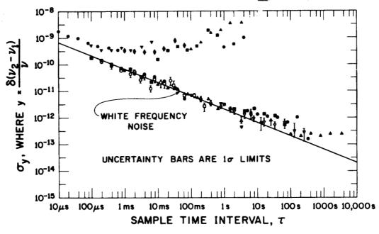
Frequency fluctuations versus sample time interval of (a) Beat between two free running He-Ne lasers (upper set of measurement points). (b) Beat between two He-Ne lasers, each independently controlled by a methane absorption cell. (Lower set of measurement points).
