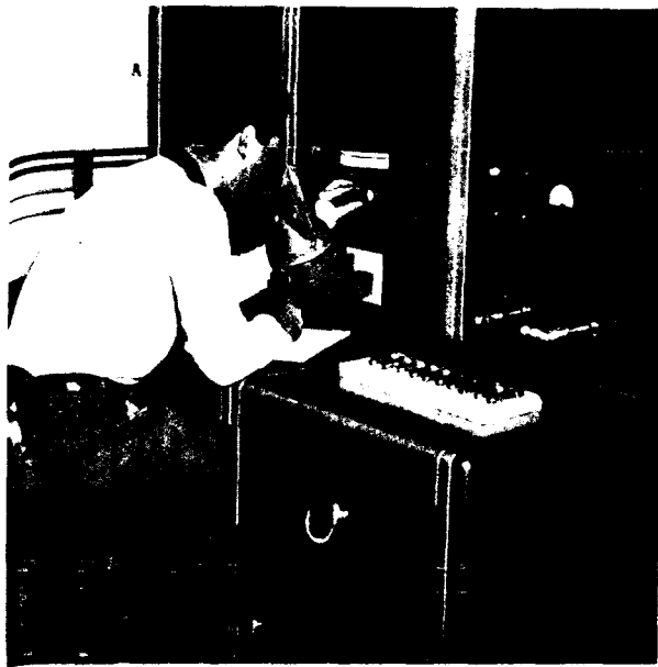
Eugene Amrine uses the new NBS high-frequency piston attenuator to calibrate the unknown inserted in the lower-right panel.
