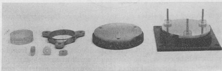
Fig. 7(a and b)—Mounting for cylindrical quartz plate (assembled and disassembled).
