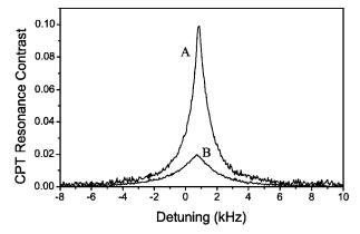
Fig. 2. CPT resonance for excitation on A, the  $D_1$  transition and B, the  $D_2$  transition with a resonant laser intensity of 160  $\mu$ W/cm<sup>2</sup>.
