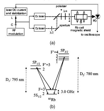
Fig. 1. Experimental setup for the comparison of the CPT resonances for excitation when the  $D_1$  and the  $D_2$  transitions are used.
