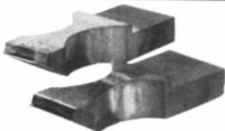
Kentanium jaws after pinching and sealing over 215,000 tubes. Note the small amount of wear on this set.
