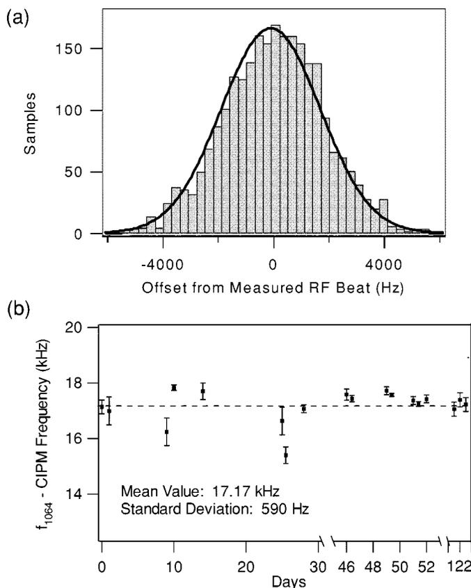
Fig. 3. (a) Histogram of 1 s counts of the sum frequency of the two beats measured at 532 and 1064 nm. The  $1\sigma$  uncertainty is 1.8 kHz. (b) Summary of measurement of one-half the  $a_{10}$  frequency ( $f_{1064}$ ) plotted with respect to the CIPM recommendation of 281 630 111 740 kHz. The +17.2 kHz average of all measurements is indicated by the dashed line.
