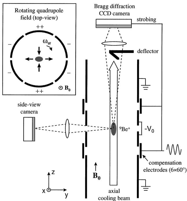
FIG. 1. Schematic side view of the cylindrical trap with real-space imaging optics and Bragg diffraction detection system. Cross section of the rotating quadrupole field (in the  $x$ - $y$  plane) is shown in the inset.
