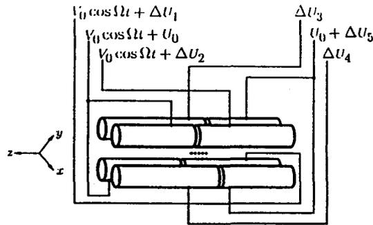
Figure 1: Linear rf trap. A rf voltage  $V_0 \cos(\Omega t)$  is applied to the four segments of two opposing trap rods. The two other rods are kept at rf ground. The voltages  $\Delta U_1$  to  $\Delta U_5$  allow for compensation of stray and patch fields. The diameter of the trap rods is 1.59 mm. See text for further explanation.
