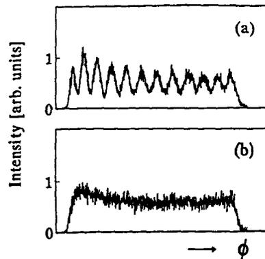
Figure 4: Polarization-sensitive detection of the scattered light (unnormalized): (a)  $\pi$ -polarized scattered light, showing interference, (b)  $\sigma$ -polarized scattered light, showing no interference (see text for explanation)
