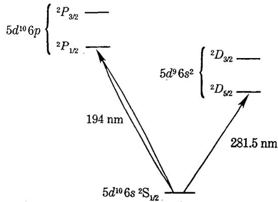
Fig. 2. - Simplified optical energy level diagram for  $\text{Hg}^+$ . The lifetime of the  $^2D_{5/2}$  level is about 0.1 s which would give a natural linewidth of approximately 2 Hz on the electric-quadrupole  $^2S_{1/2} \rightarrow ^2D_{5/2}$  transition. By observing the presence or absence of fluorescence from the  $^2S_{1/2} \rightarrow ^2P_{1/2}$  transition, the quadrupole «clock» transition can be detected with 100% efficiency.
