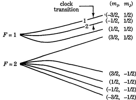
Fig. 1. - Hyperfine energy levels (not drawn to scale) of the  ${}^9\text{Be}^+ 2s \ ^2S_{1/2}$  ground state as a function of magnetic field. At  $B = 0.8194$  T the 303 MHz clock transition is independent of magnetic field to first order.
