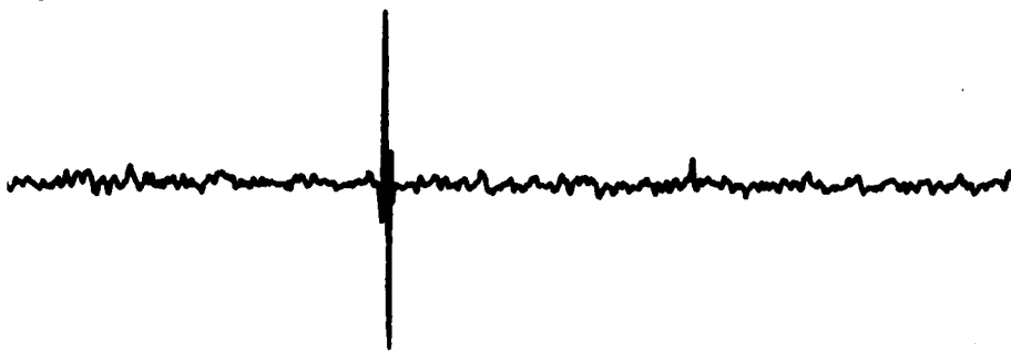
Figure 3. The third derivative saturated absorption signal of the OCS P(27) line at 3.4 \mu\text{m} . The linewidth is less than 200 kHz.
