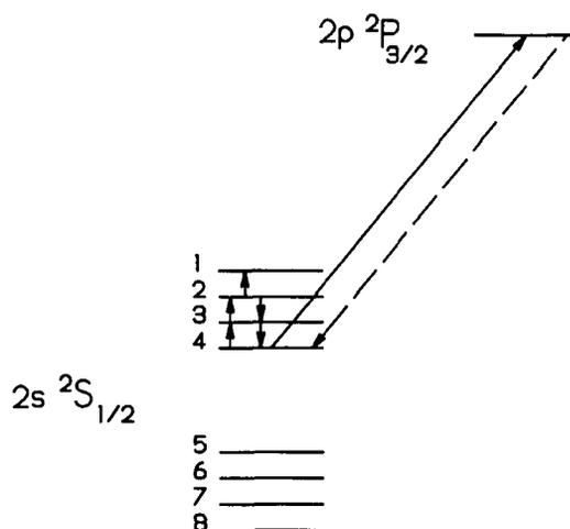
Fig. 2. Level diagram showing the transitions involved in the state preparation and detection for the  ${}^9\text{Be}^+$   $2s\ 2S_{1/2}$  ( $m_I = -3/2, m_J = 1/2$ ) to ( $m_I = -1/2, m_J = 1/2$ ) (state 1 to 2) transition in the electronic ground state.
