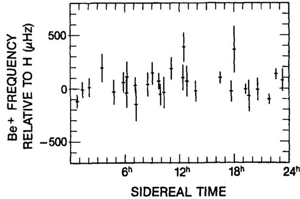
Fig. 4. The  ${}^9\text{Be}^+$  transition frequency with respect to sidereal time. The orientation of the trap magnetic field (which defines the quantization axis for the  ${}^9\text{Be}^+$  ions) with respect to the fixed stars varies due to the rotation of the Earth. A daily variation of the frequency would indicate a violation of local Lorentz invariance. (From ref. [18].)
