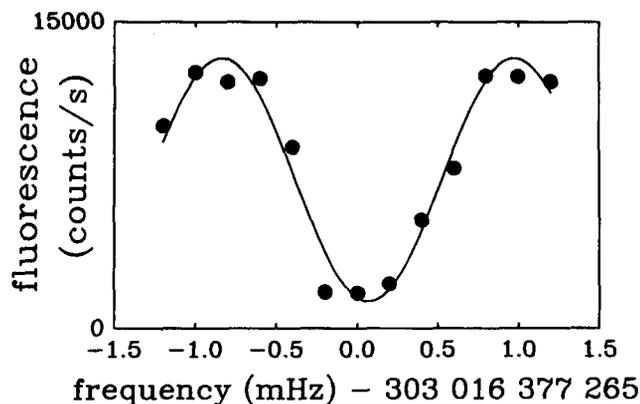
Fig. 3. Example of a 303 MHz  ${}^9\text{Be}^+$  hyperfine resonance obtained by Ramsey's method of separated oscillatory fields. The time between the two rf pulses was 550 s. The width of the resonance is 0.9 mHz (0.0009 Hz). (From ref. [4].)
