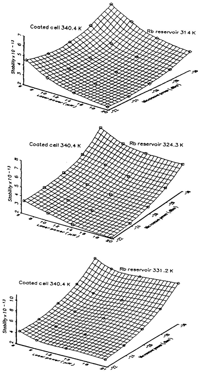
Fig. 4. Evaluated stability vs. microwave and optical power. The stability is calculated from measured noise current and discriminator slope;  $\sigma_y(\tau) \equiv [1/\sqrt{2}] \cdot [i_n/D\nu_o] \cdot \tau^{1/2}$ , [ 14].
