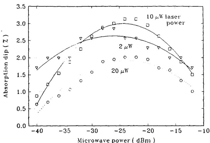
Fig. 3. Microwave resonance strength ( $\Delta I/I$ ) as a function of microwave power at the synthesizer. The cell is at room temperature. The maximum signal (3%) is vastly higher than any lamp pumped standard even operated at 70°C.
