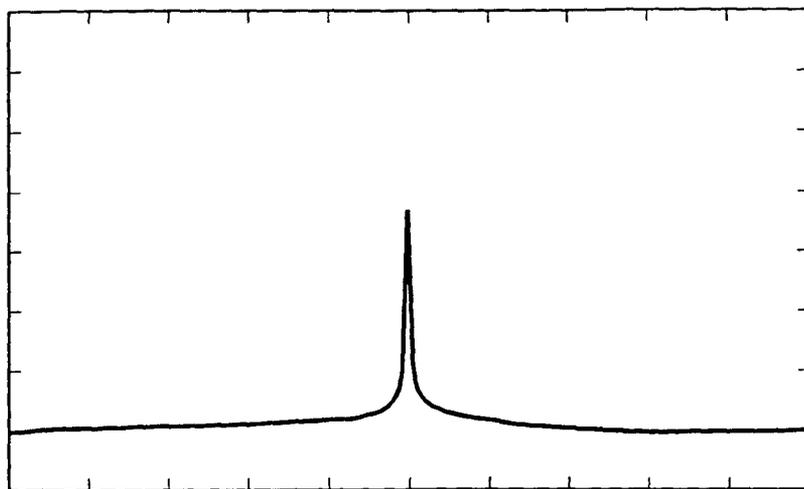
Fig. 2. Dicke narrowed lineshape observed in an evacuated, wall-coated cell in a  $TE_{011}$  cavity. The cell is at room temperature. The measured linewidth (FWHM) is 87 Hz.
