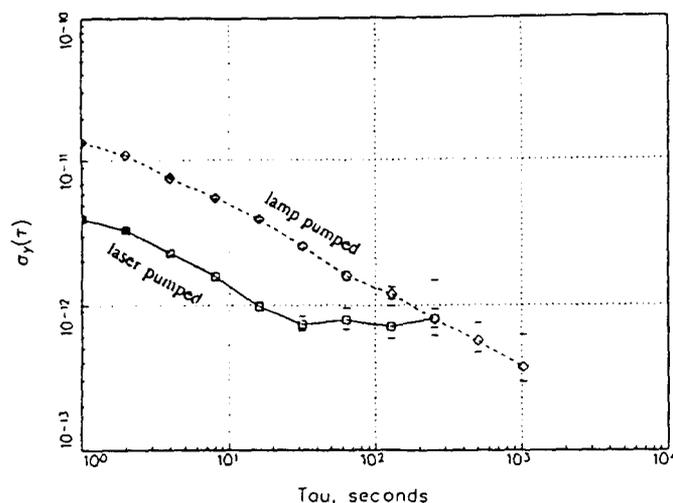
Fig. 1. Frequency stability of commercial standard with lamp pumping and laser pumping. The flicker floor seen in the laser data at times greater than about 20 s is the result of unregulated laser amplitude.
