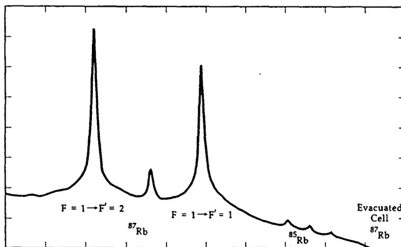
Fig. 6. Saturated absorption signals obtained in an evacuated <sup>87</sup>Rb cell. A small residual of <sup>85</sup>Rb can be seen as the closely spaced triplet in the lower right of the plot.
