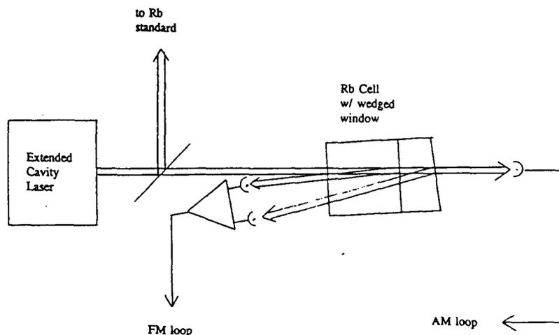
Fig. 5. Schematic for obtaining saturated absorption spectra from very simple layout.
