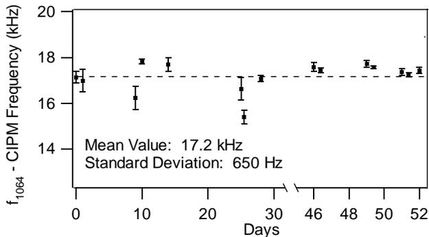
FIG. 4. Summary of measurement of one-half the  $a_{10}$  frequency ( $f_{1064}$ ) plotted with respect to the CIPM recommendation of 281 630 111 740 kHz. The +17.2 kHz average of all measurements is indicated by the dashed line.
