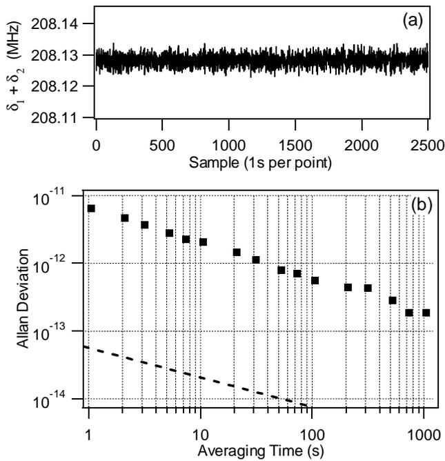
FIG. 3. (a) Time record of the counted sum of the heterodyne beats at 1064 and 532 nm, which represents a measurement of the 282 THz optical frequency of  $f_{1064}$ . (b) The squares are the Allan deviation of the optical frequency computed from the above time record. For comparison, the dashed line is the measured Allan deviation between “JILA East” and “JILA West” Nd:YAG/I<sub>2</sub> systems.
