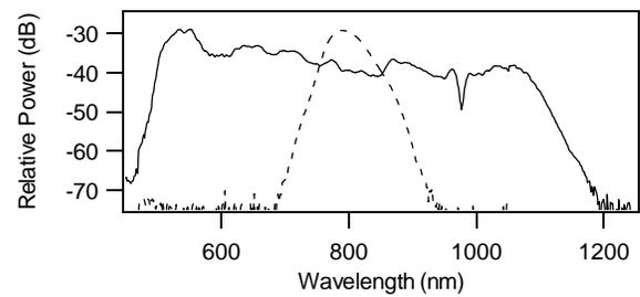
FIG. 2. Output spectrum from the silica microstructure fiber (solid line). The spectrum directly from the laser is indicated by the dashed line.
