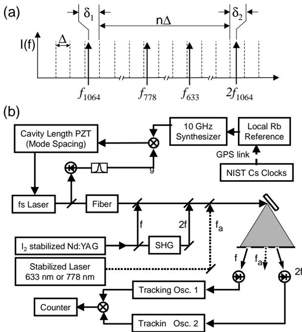
FIG. 1. (a) The femtosecond laser comb spans an octave such that the optical frequency  $f_{1064}$  can be expressed as an integer multiple of the comb spacing  $\Delta$  plus small measured offsets  $\delta_1$  and  $\delta_2$ . (b) Apparatus used for measurement of the optical frequencies in terms of the cesium microwave standard.
