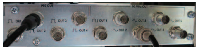
Figure 7. Back panel of a GPSDO with multiple output signals.
