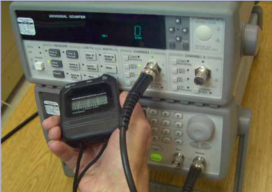
Figure 14. Using the start-stop button of the stopwatch to start the counter.
