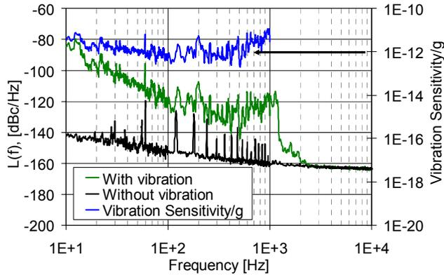
Figure 3(a). PM noise floor of the measurement system measured with and without vibration using a semi-rigid cable. A random vibration profile of acceleration PSD  $0.5 \text{ mg}_{\text{rms}}^2/\text{Hz}$  for offset frequencies 10 Hz to 1200 Hz was used.
