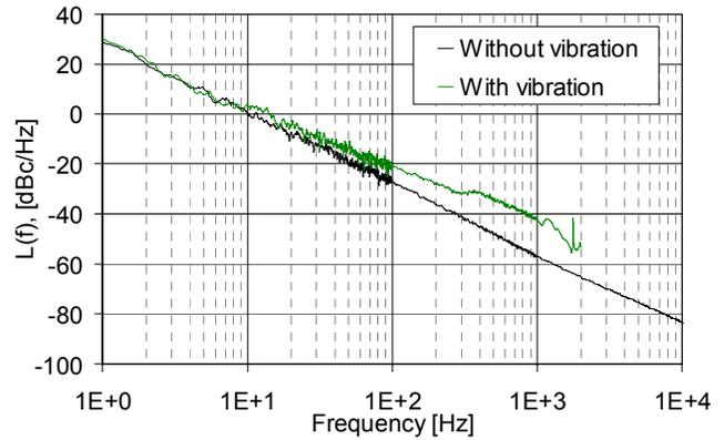
Figure 8(a). PM noise of the DRO with and without vibration along the z-axis. A random vibration profile of acceleration PSD  $0.5 \text{ mg}_{\text{rms}}^2/\text{Hz}$  for offset frequencies 10 Hz to 1500 Hz was used.
