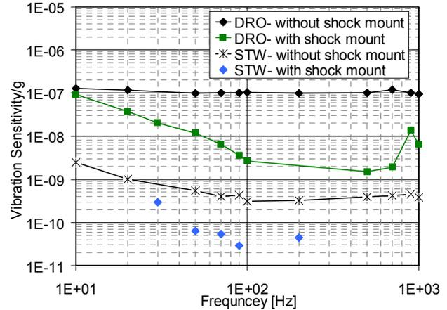
Figure 12. Improvement in vibration sensitivity using shock mount.
