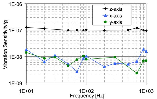
Figure 8 (b):. Vibration sensitivity of a DRO.  $a = 0.5 \text{ g}_{\text{peak}}$  was used for sinusoidal dwell frequencies.
