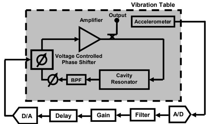
Figure 13 (a). Block diagram of experiment to suppress vibration-induced PM noise in ACCRO.
