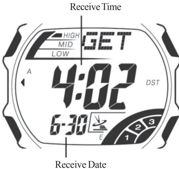
Figure 7. RCC display indicating the date and time of the last synchronization.
