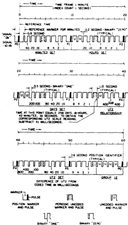
Time-scale representation of carrier level-shift modulation. BCD code gives time, day, and difference between WWVB and UT2 time scales.
